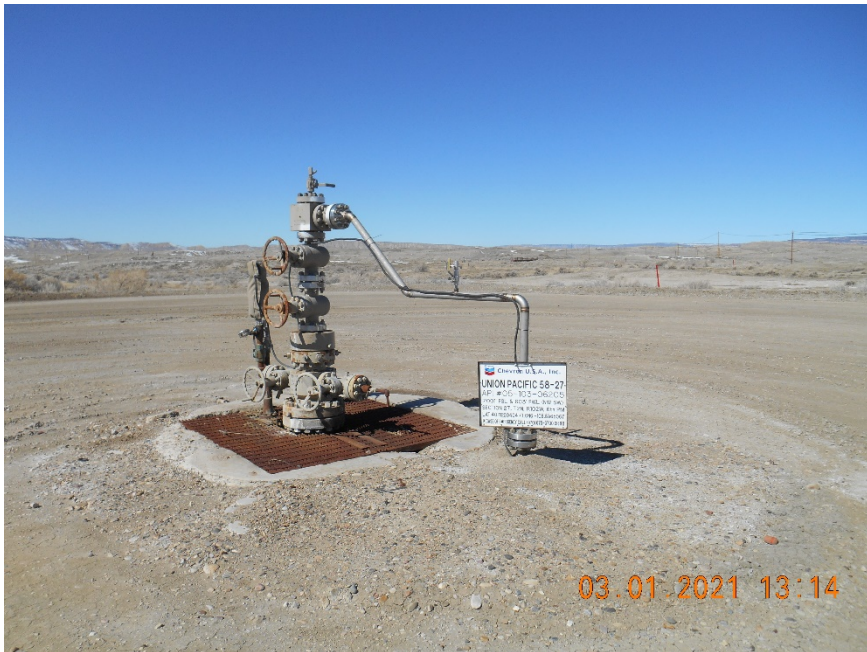
Injection wellhead
