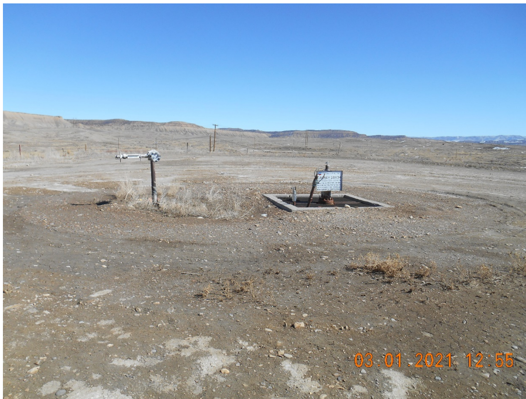
Injection wellhead – Temporarily abandoned
