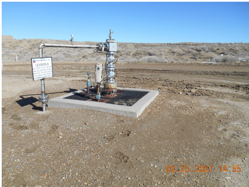
Injection wellhead
