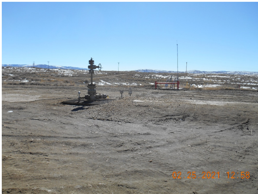
Injection wellhead – Temporarily abandoned
