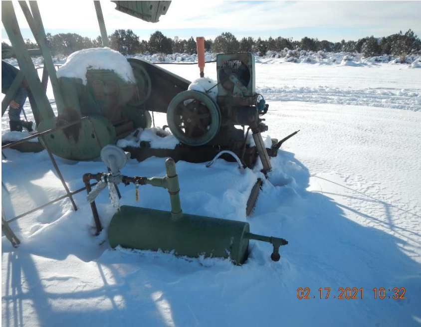
Natural gas powered prime mover and drop out tank for supply gas.
