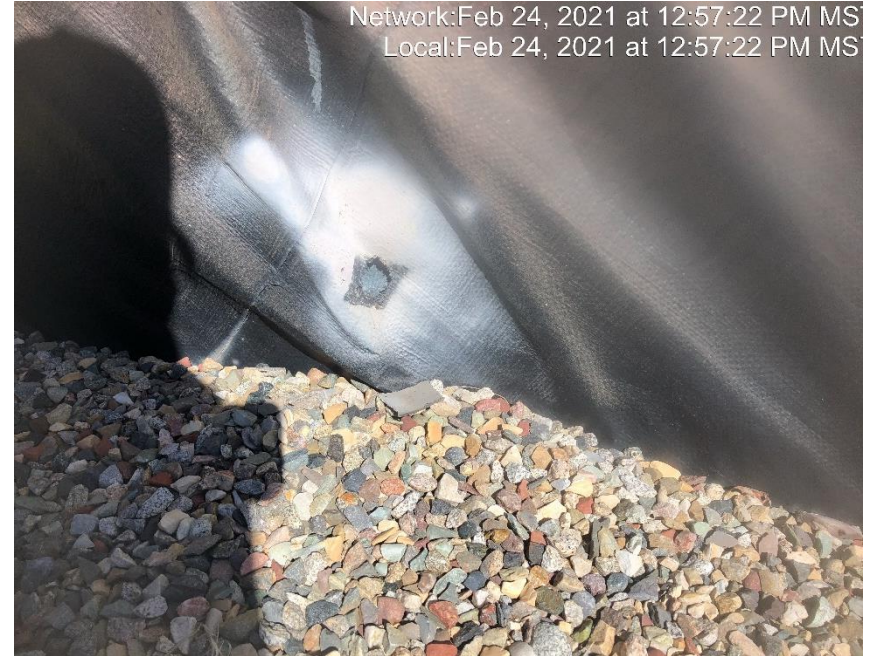
Photo #2963 Multiple holes in tank containment liner
