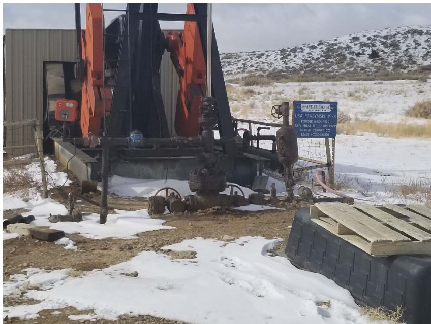
Photo 2. No bradenhead access apparent.
