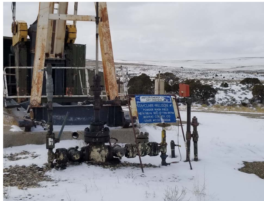
Photo 2. No bradenhead access apparent.
