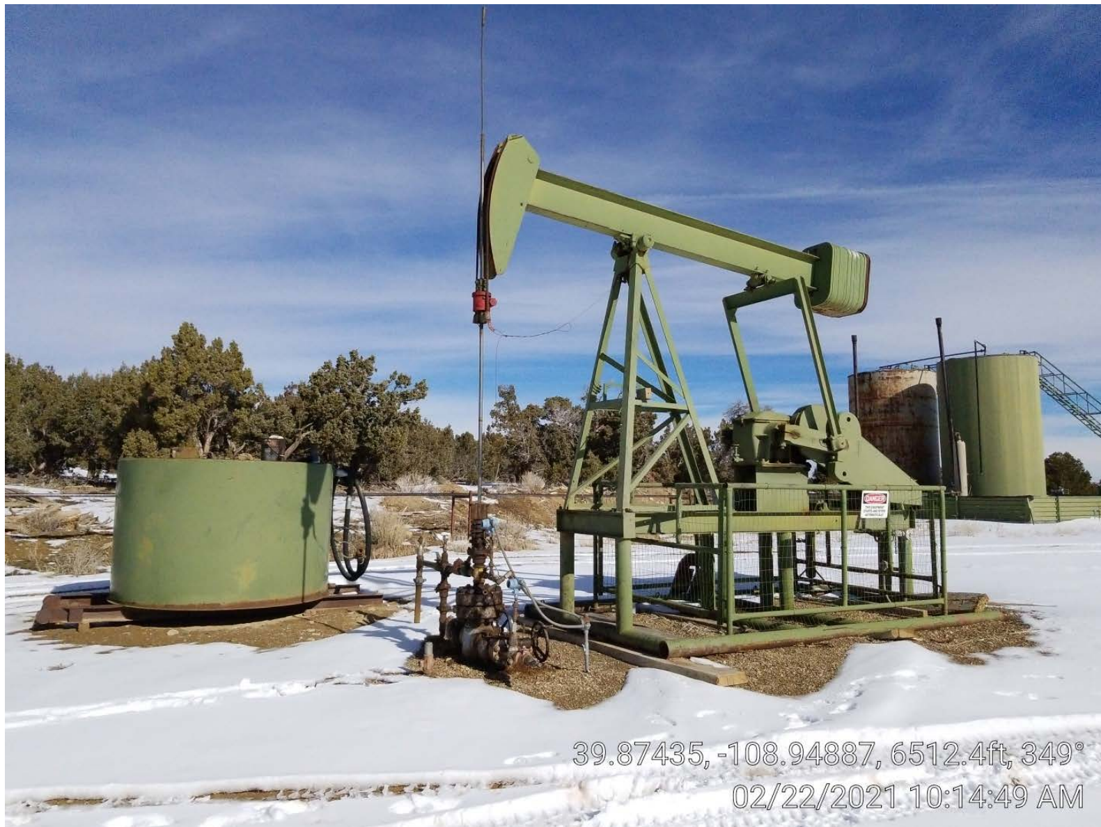
Photo 2. Tanks & pump jack.
