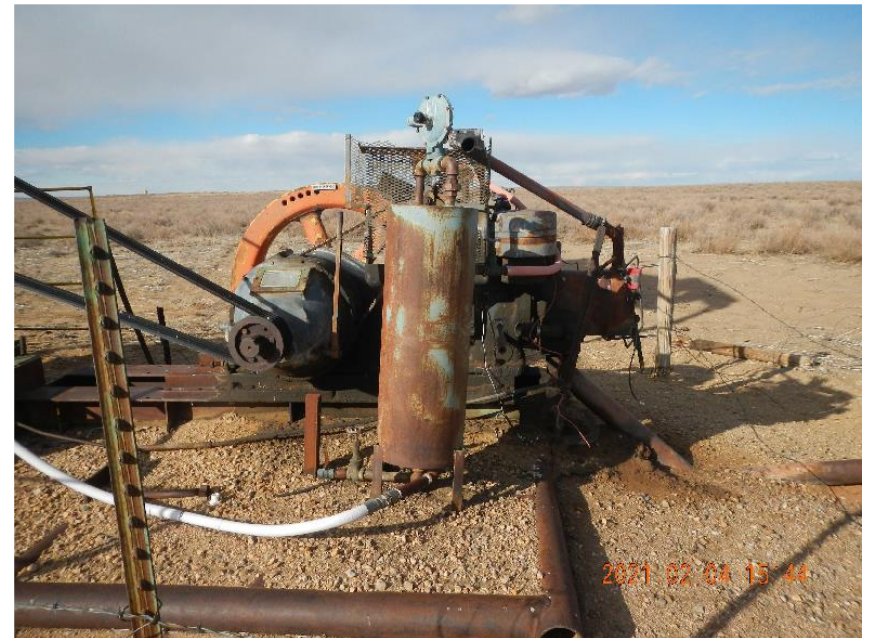
Photo 4: Gas dryer vessel with gas operated prime mover in background. Stained soil visible around prime mover.
