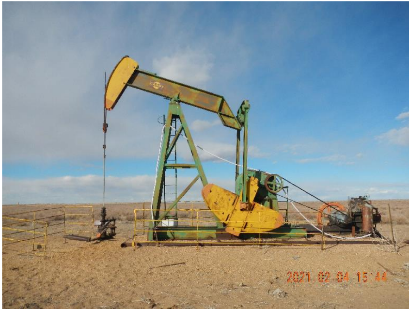
Photo 3: View of pumping unit.
