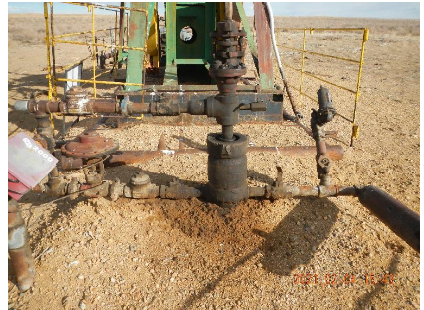
Photo 2: View of wellhead. Stained soil visible around base. Production flowline off L side of well tree.
