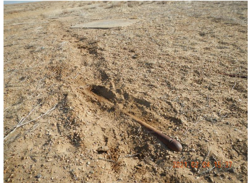
Photo 2: Flowline riser at site E of pumping unit.
