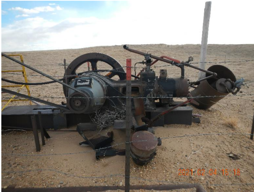
Photo 7: Gas powered prime mover.
