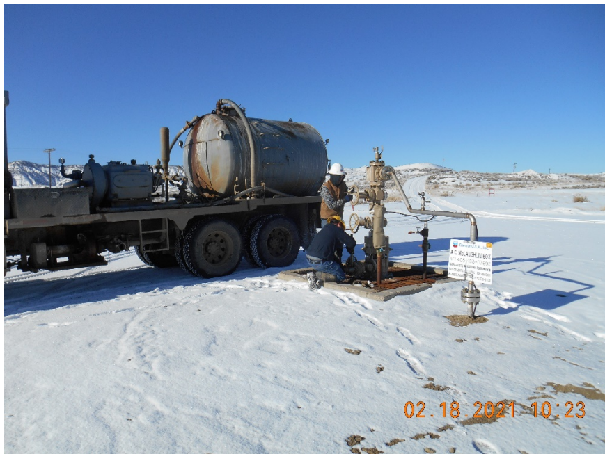
Injection wellhead
