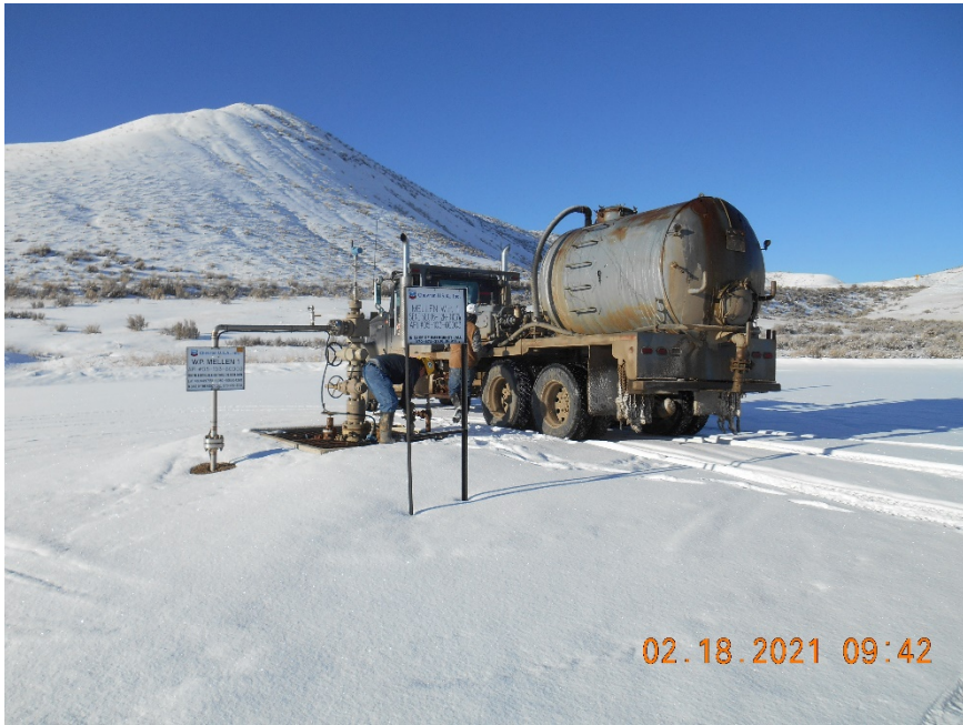
Injection wellhead
