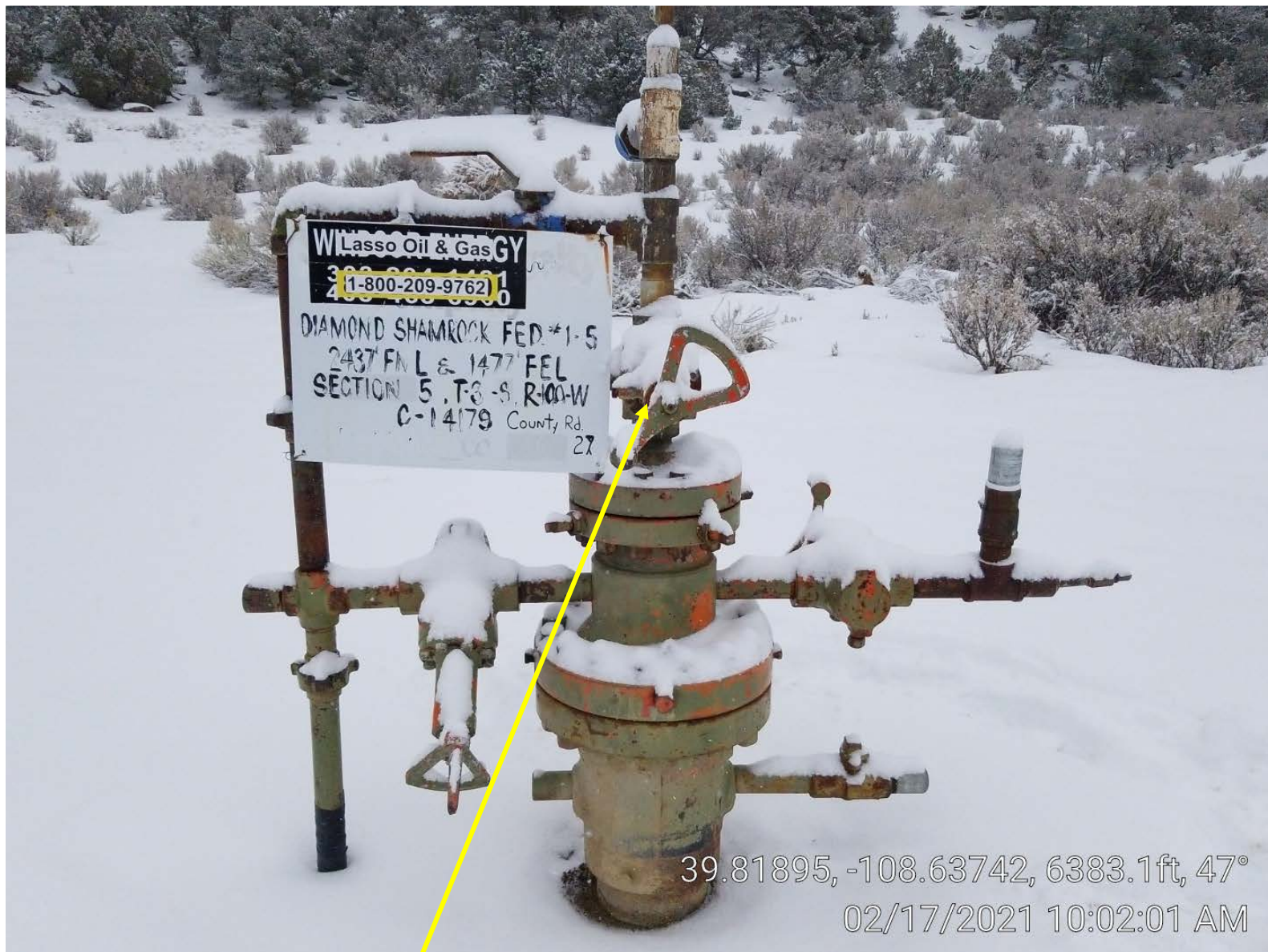
Photo 2. Well with gas leak.
