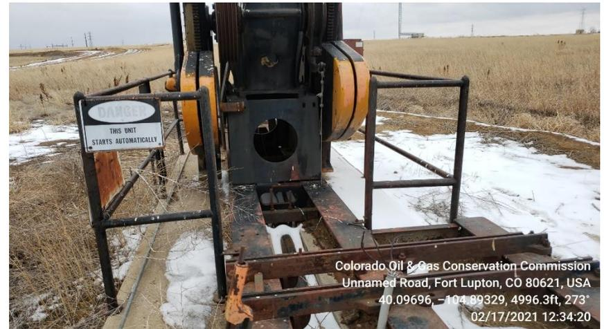
Photo 5 electric motor removed from Pump jack
