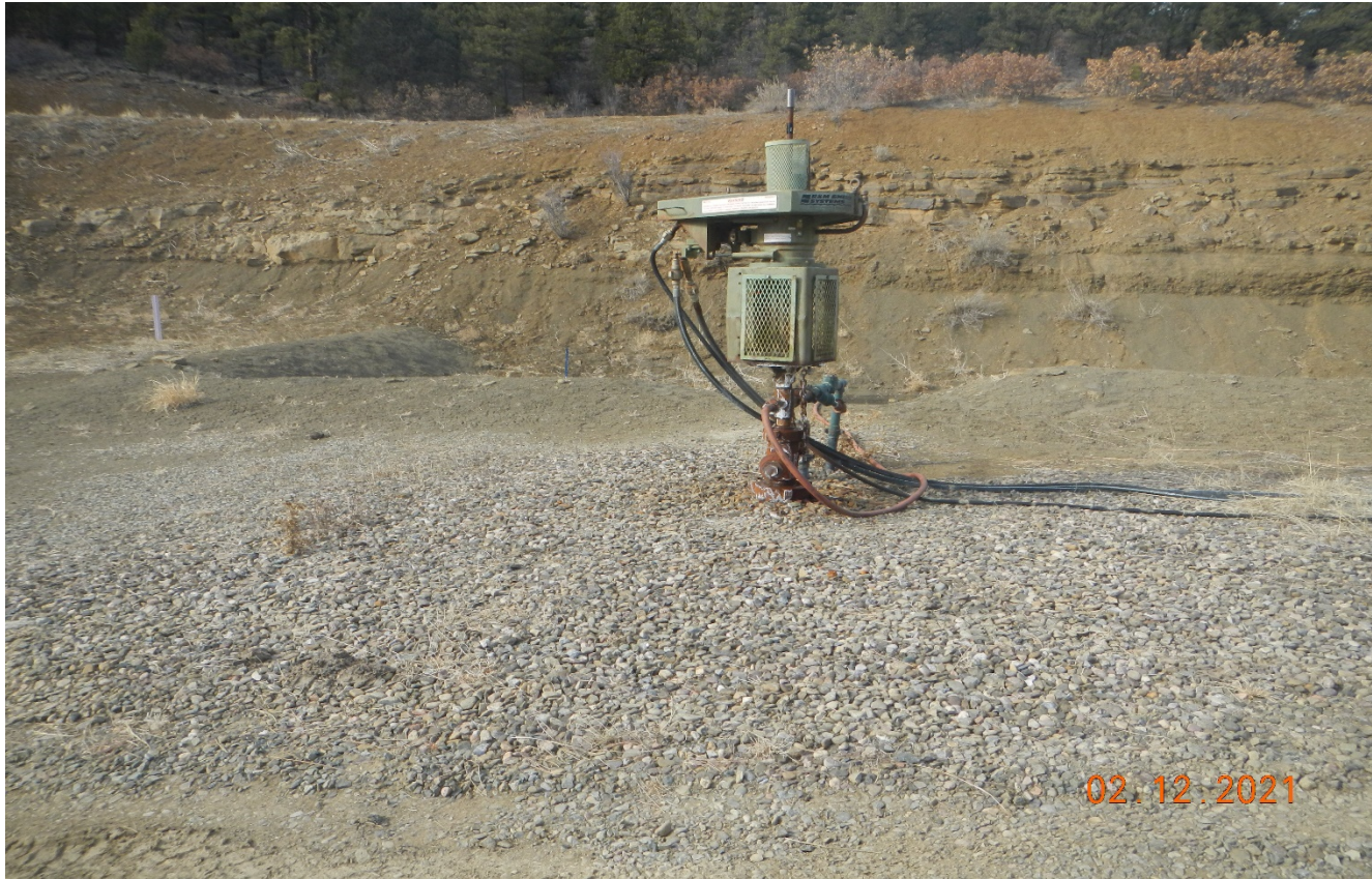
Photo 2. The dripping water leak at the wellhead has been repaired.
