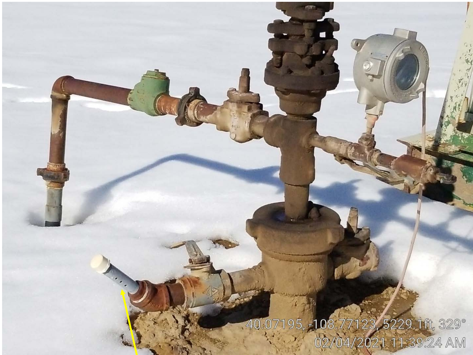
Photo 2. Well with gas leak.
