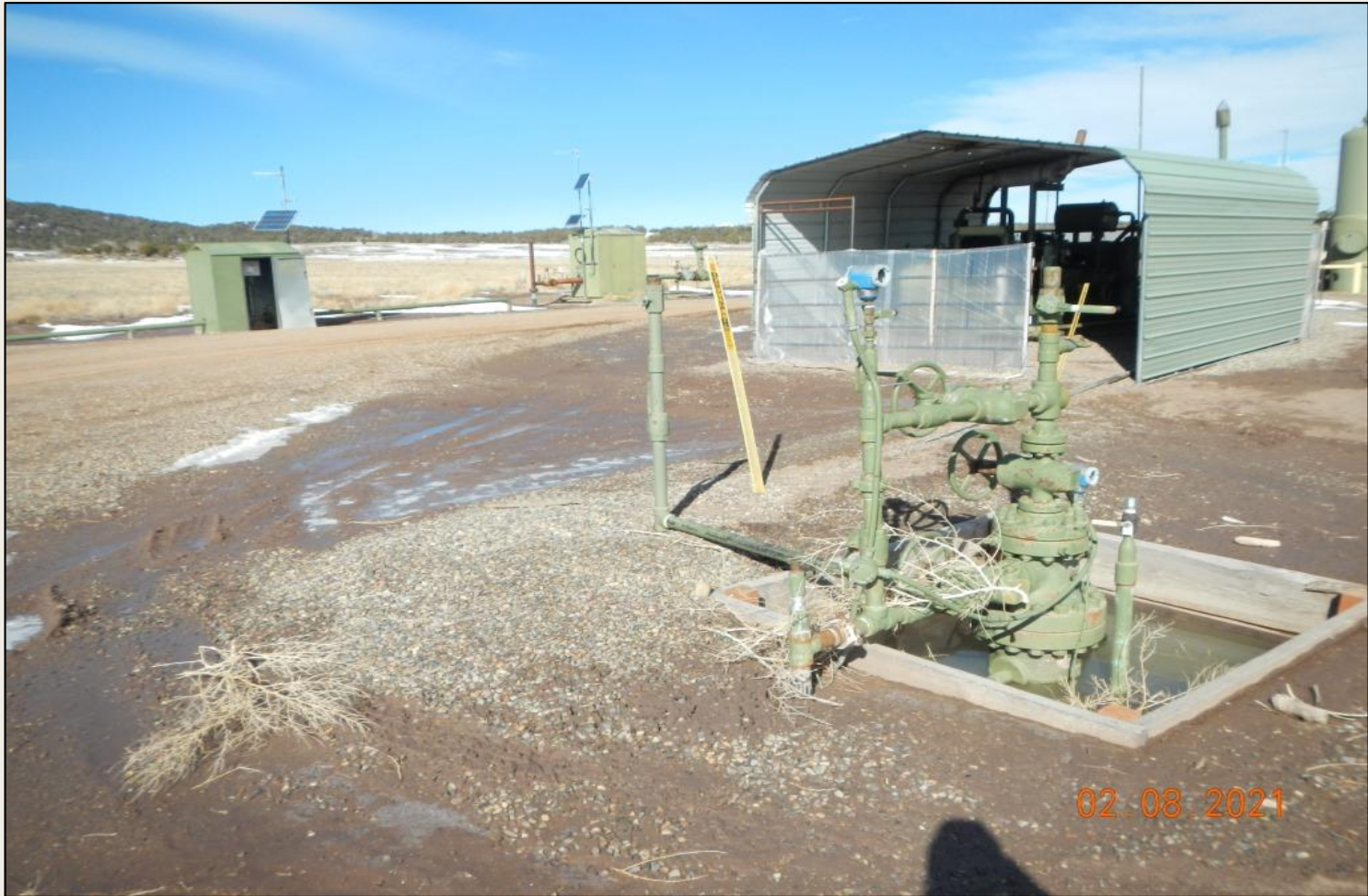
Photo 3. View of kochia debris stuck around wellhead.
