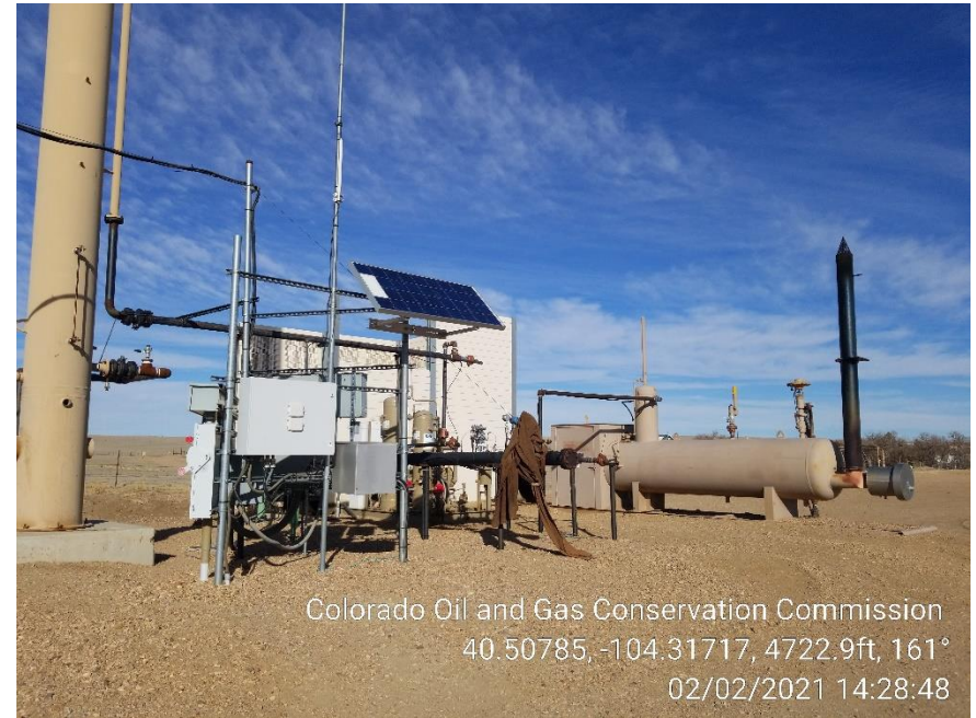
Photo 2 – Separator, VRU and VRT
