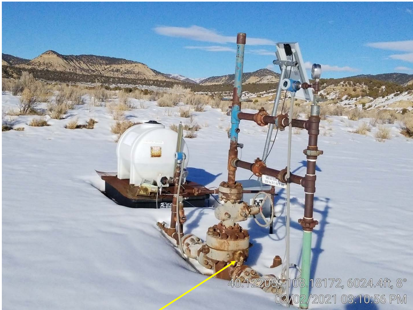
Photo 3. Well. Gas leak.
