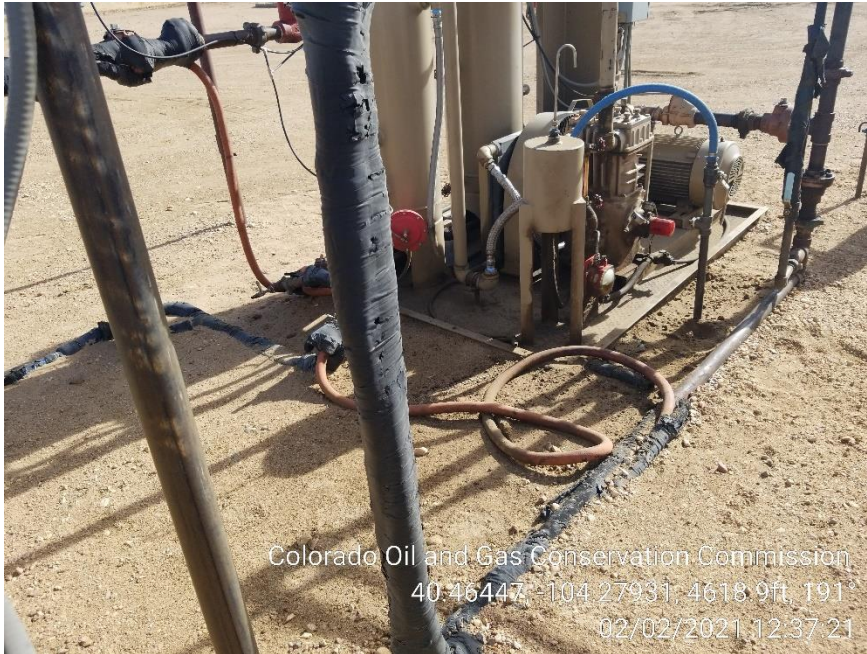
Photo 9 – VRU – Stained Soil
