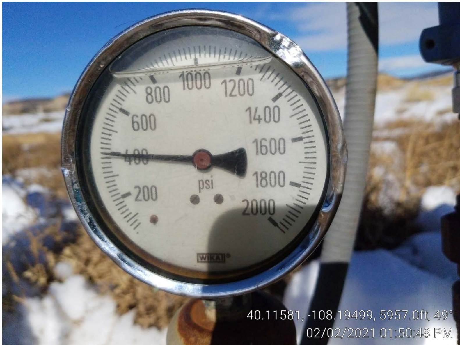
Photo 3. Casing gage.
