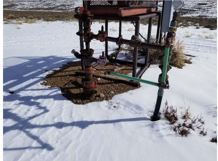
Photo 2. No bradenhead access apparent.
