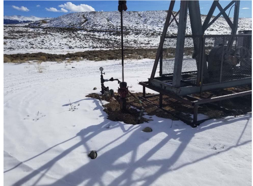
Photo 2. No bradenhead access apparent.
