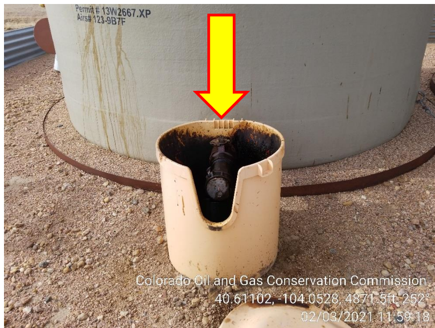
Photo 15 – Loadline Bucket at Produced Water Tank – Oily Waste and Lid Missing
