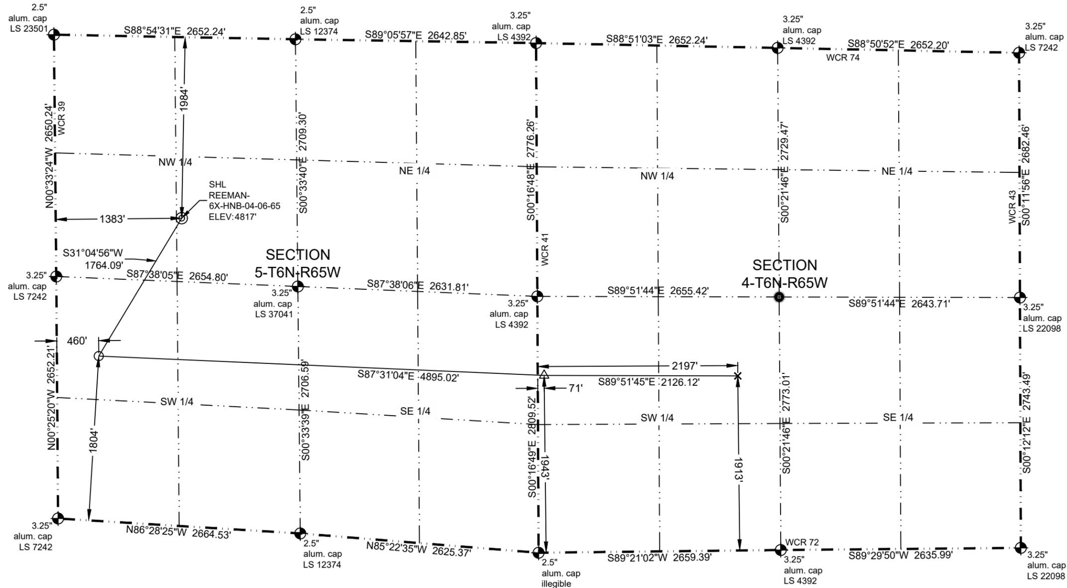
In accordance with a request from Kit Tinchler of Nickel Road Operating LLC, Sterling Land Surveyors, LLC has determined the location of the **REEMAN-6X-HNB-04-06-65** well site to be SHL: 1984' FNL and 1383' FWL, (LPL: 18.4' FSL and 460' FWL), (APL: 1943' FSL and 71' FWL), (BHL: 1913' FSL and 2197' FWL), as measured at ninety (90) degrees from the section lines of Sections 4 and 5, Township 6 North, Range 65 West of the 6th Principal Meridian, Weld County, Colorado.
