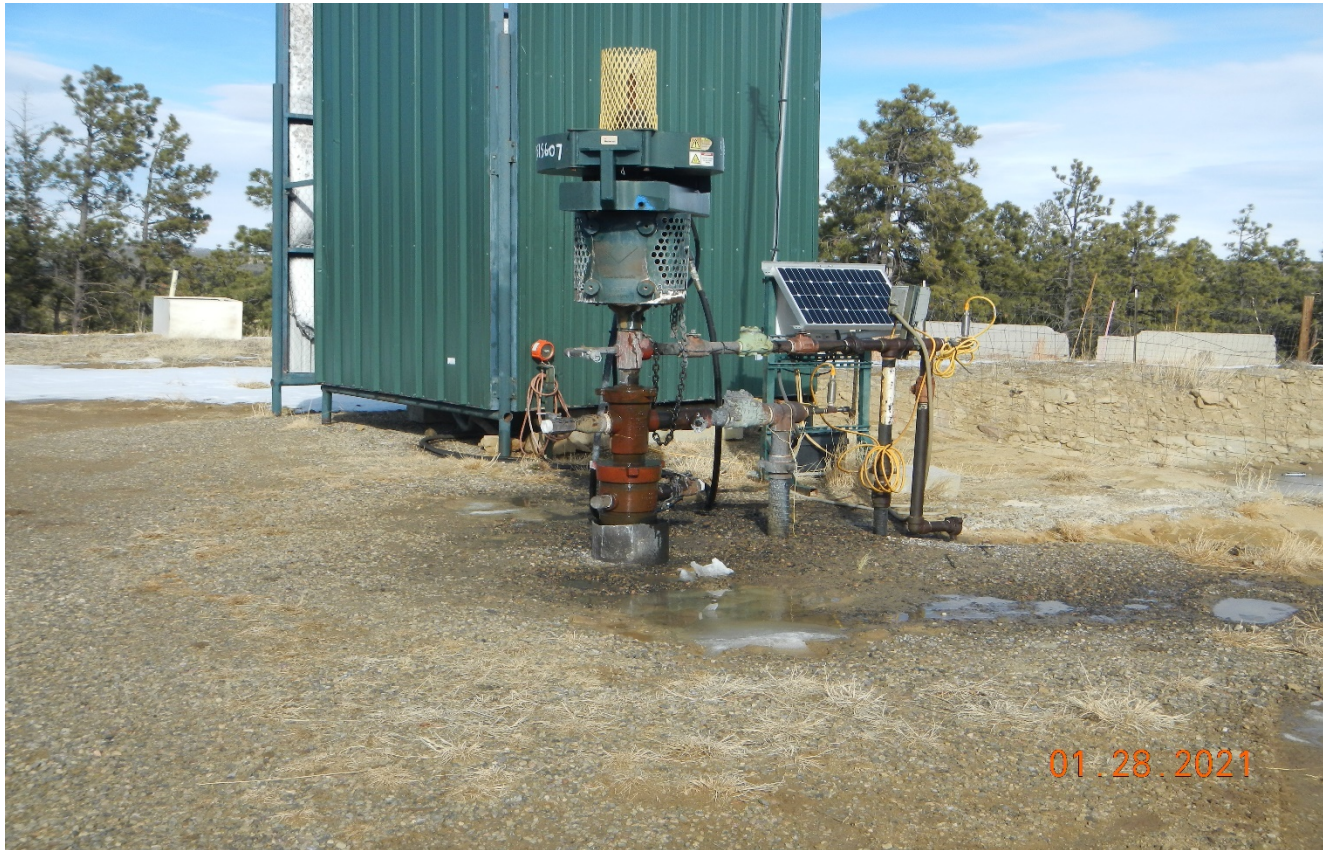
Photo 3. Facing toward the well. There is a dripping water leak at the well head.
