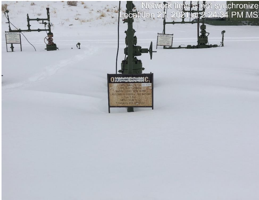
Photo #2737 Multiple wellhead signs weathered and not legible.
