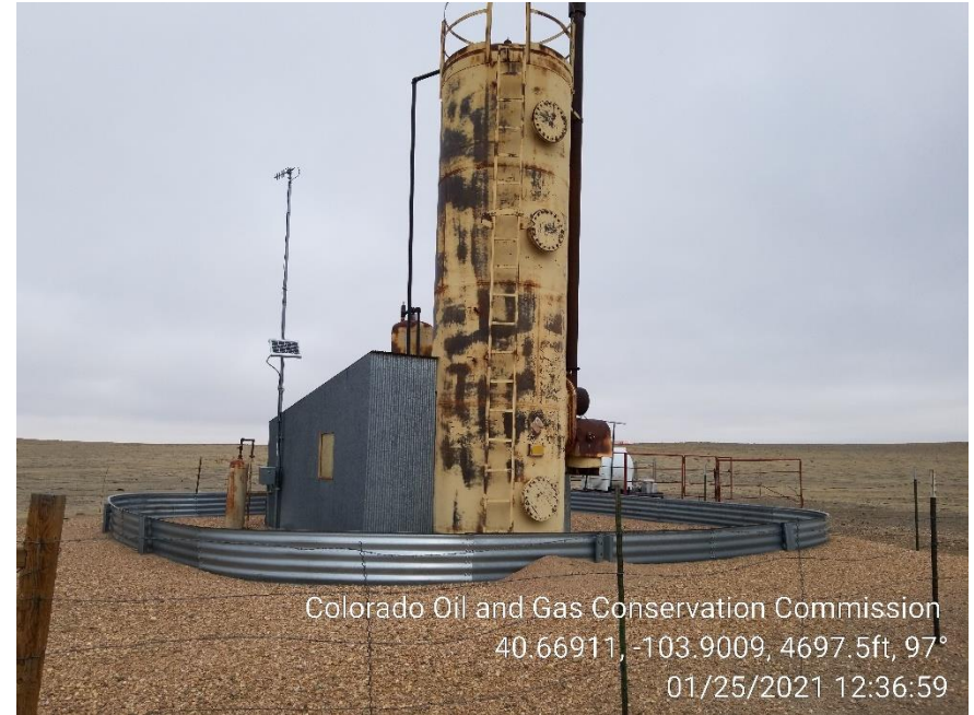
Photo 2 – Heater Treater
