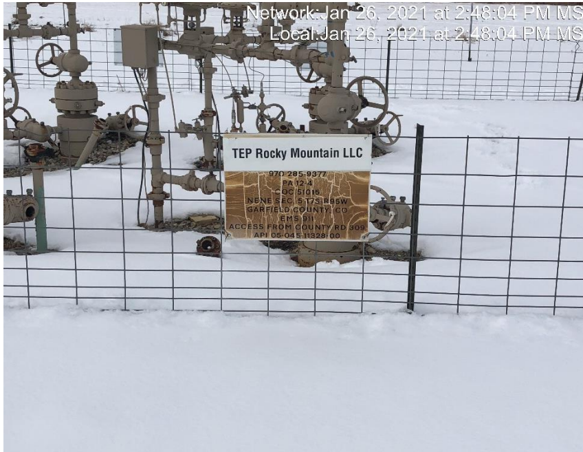
Photo #2725 Multiple wellheads signs weathered and not legible.
