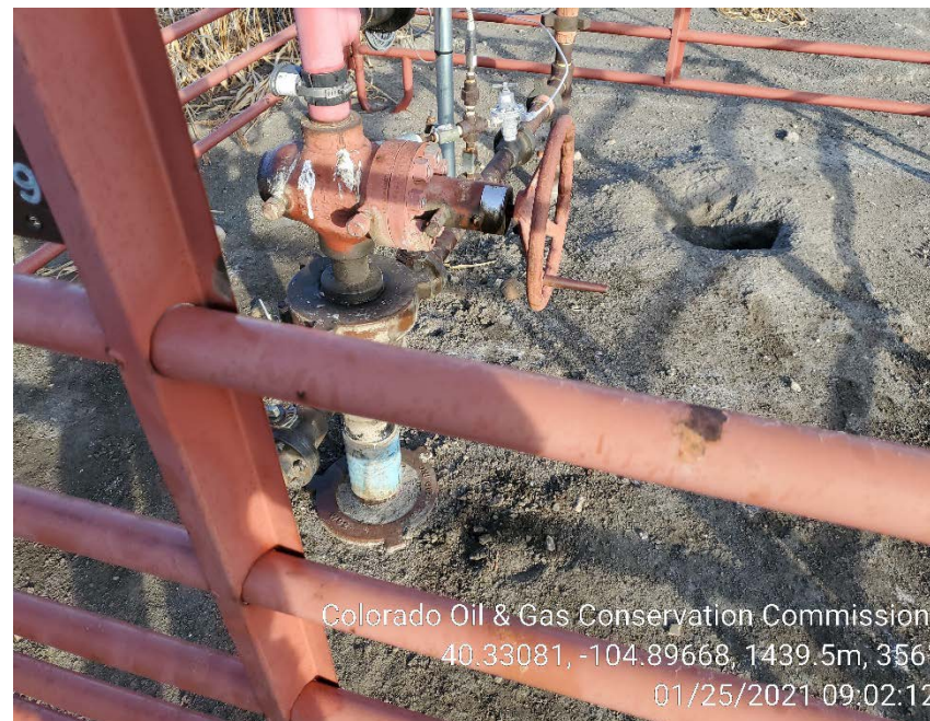
Master valve leak on 1/25/2021
