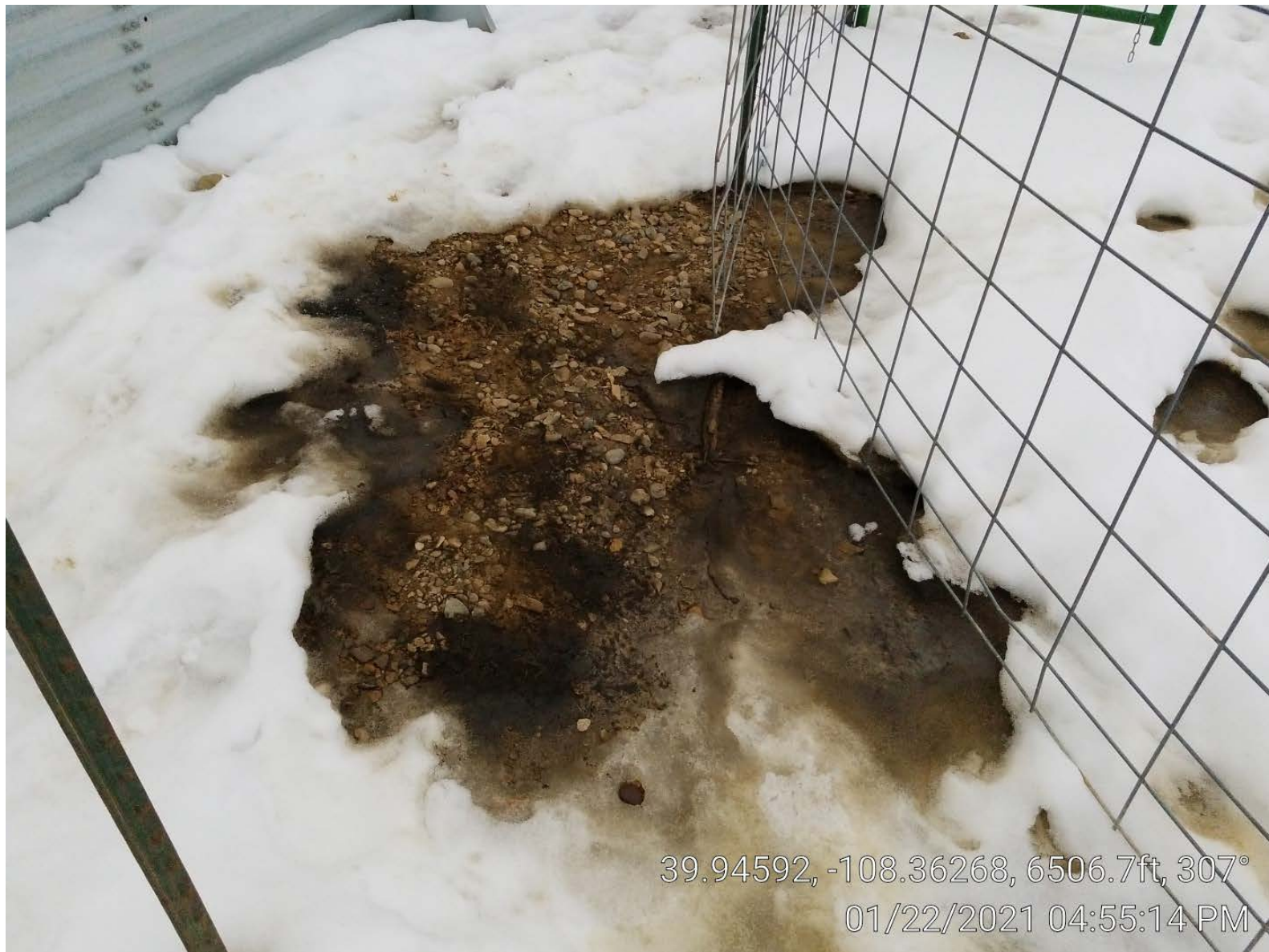
Photo 9. Stained soil outside tank battery.
