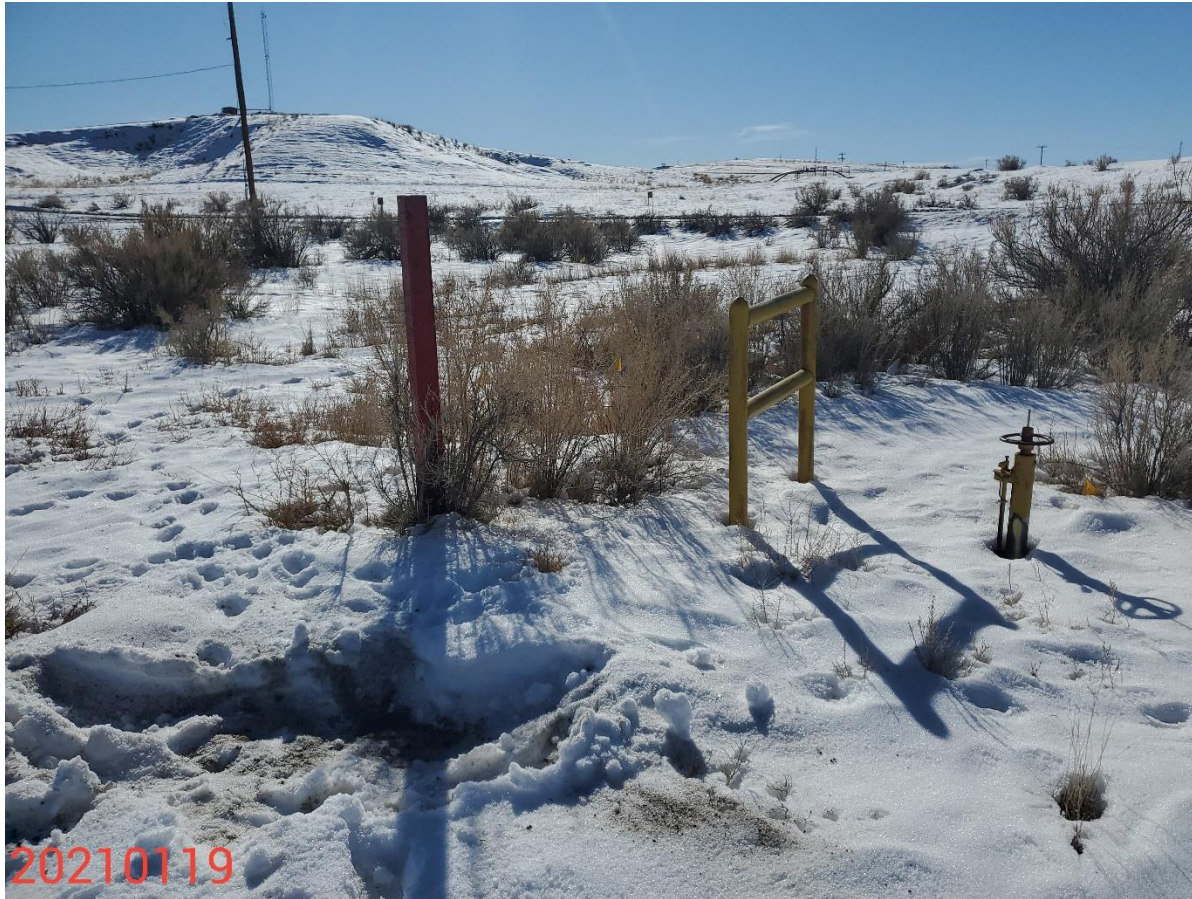
Photo 1: Photo shows PA well marker and active shut off valve.
