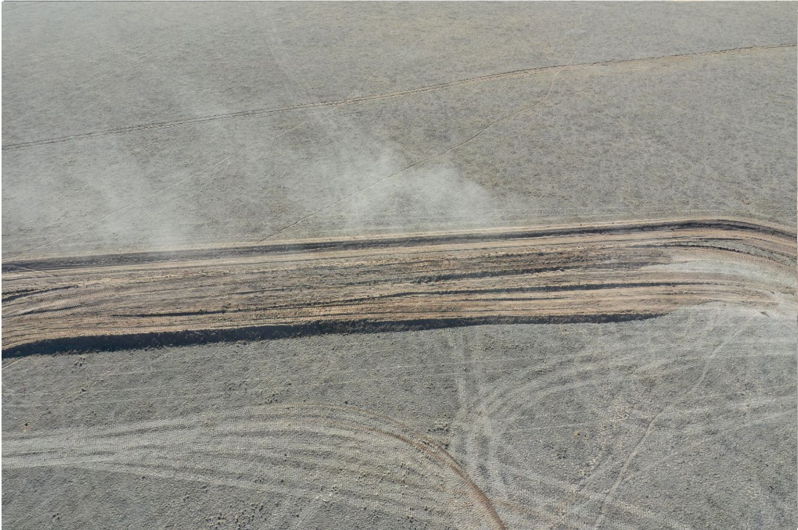
Photo 5. Drone aerial imagery illustrates the southern location, facing South. Photo illustrates the topsoil stockpile.
