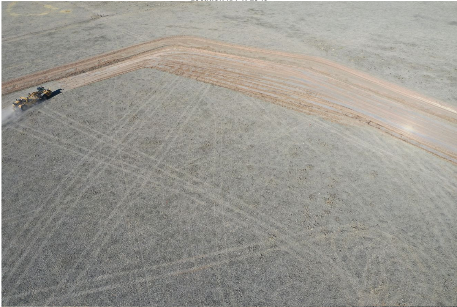
Photo 3. Drone aerial imagery illustrates the northwestern location, facing Northwest. See comments under Photo 1. Topsoil salvage operations were underway at the time of this inspection along the northern location.
