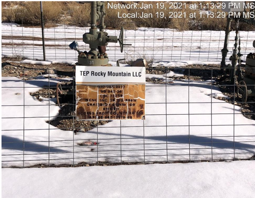
Photo #2653 Multiple wellhead signs weathered and not legible.
