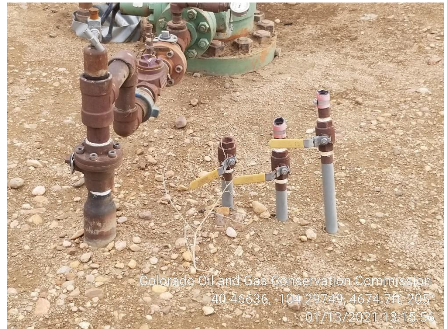
Photo 6 – Unmarked 1" Risers at Wellhead
