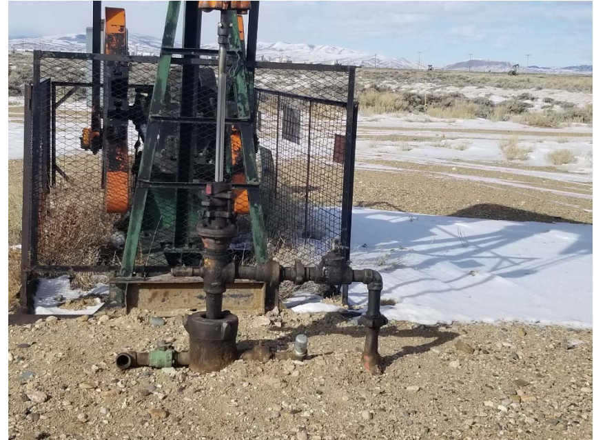
Photo 2. No bradenhead access apparent.
