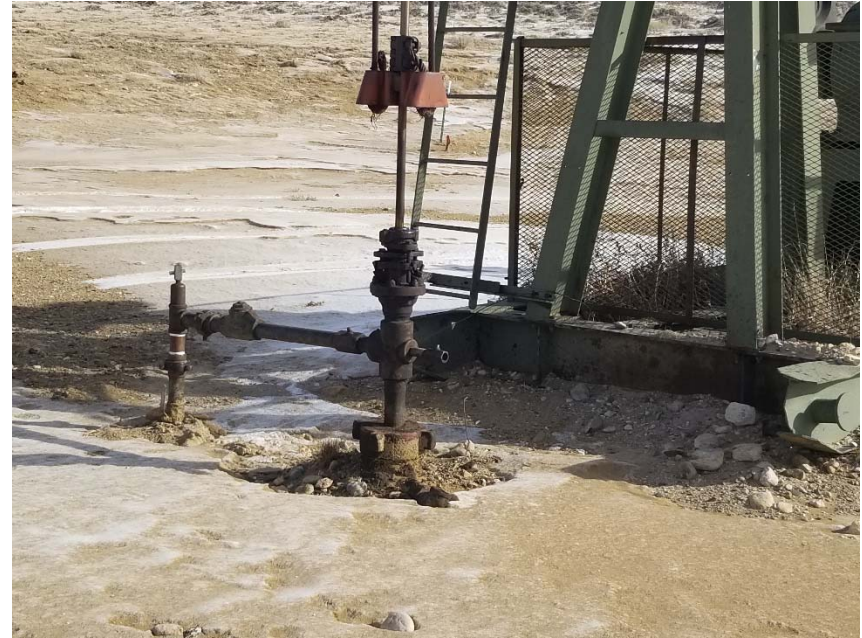
Photo 2. No bradenhead access apparent.
