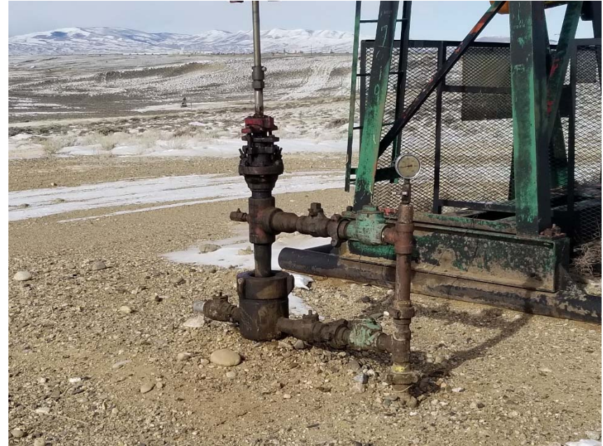
Photo 2. No bradenhead access apparent.
