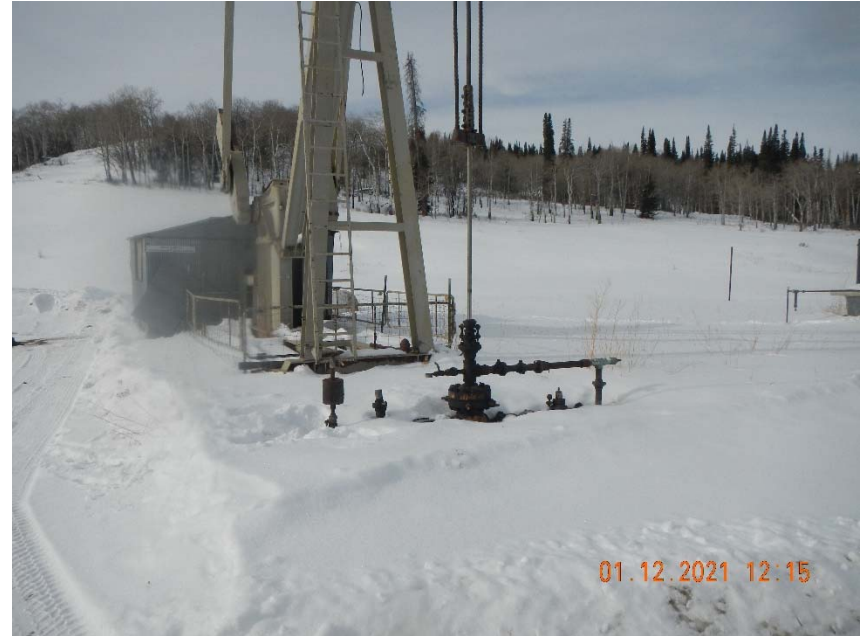
Photo 2. No bradenhead access apparent.
