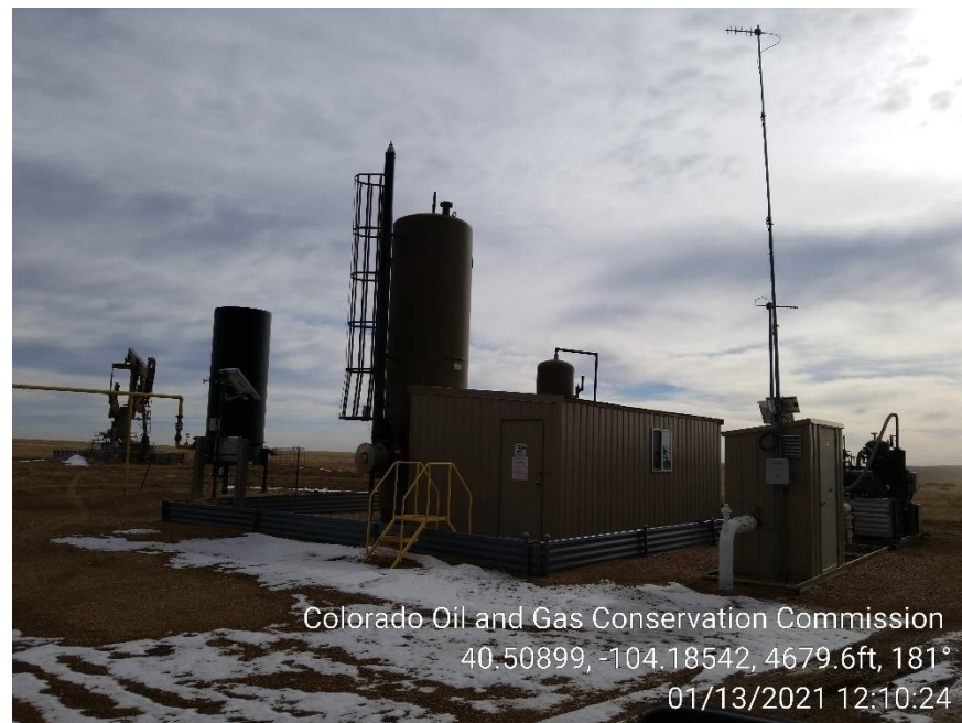
Photo 4 – Heater Treater and ECD
