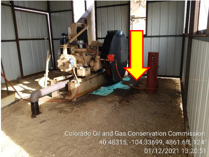
Photo 5 – Stained Soil at North Engine
