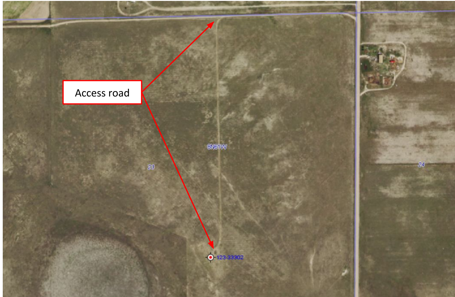
Photo 2. COGCC GISOnline aerial imagery from 2019 illustrates the access road which has not been reclaimed per Rule 1004. On 1/14/2021, Operator was commencing final reclamation activities to reclaim the above access road.
