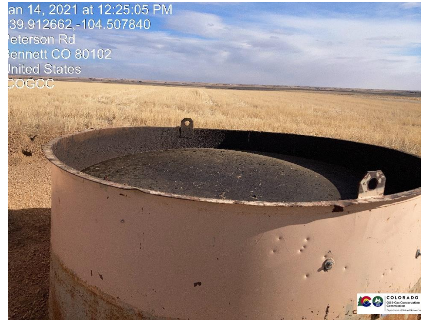
Pic 6 no netting on open top tank / hydrocarbons present
