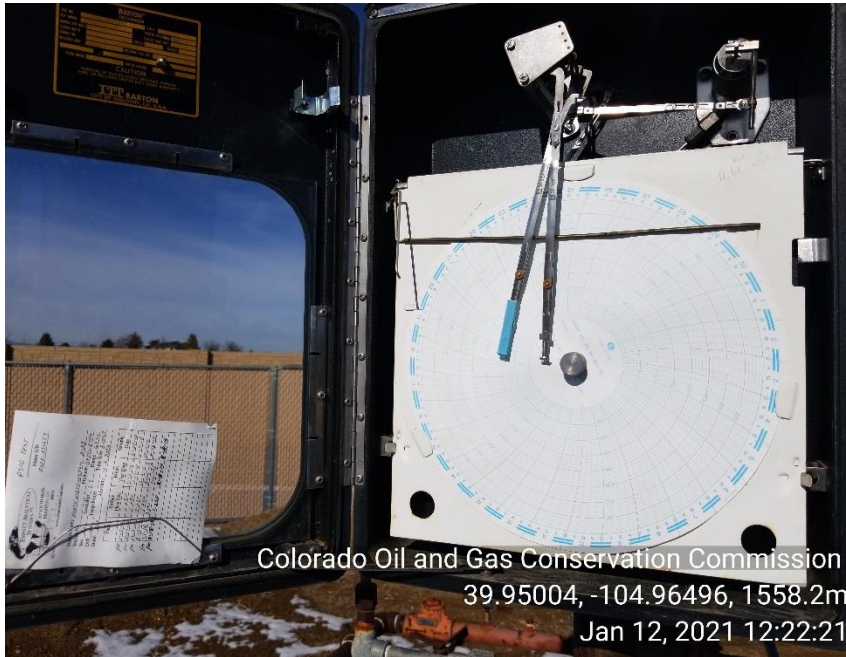
Photo 5 Calibration card out of date 2014 and gas meter does not appear to be in operation.
