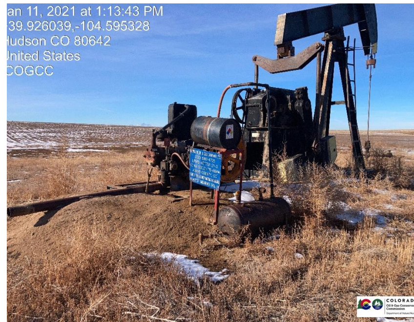
Pic 2 no BMP under chemical tank
