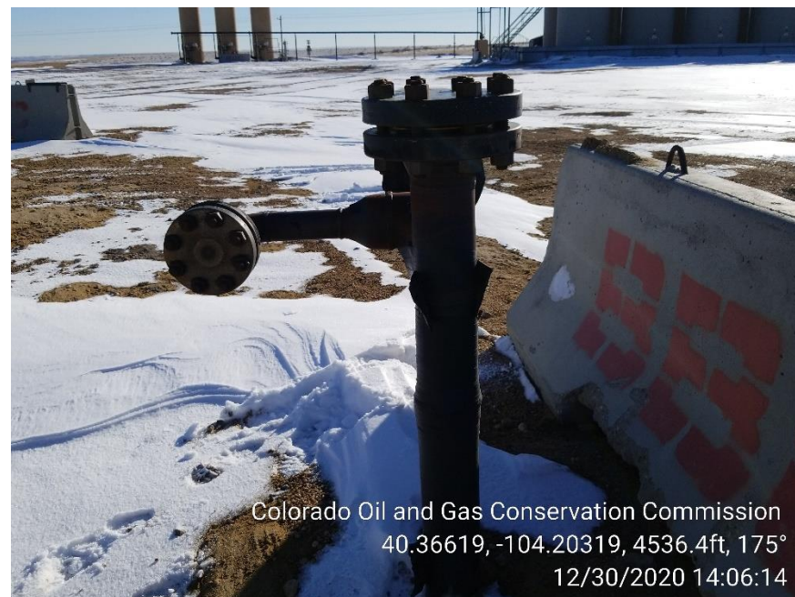
Photo 6 – Unmarked Riser at Soundwall
