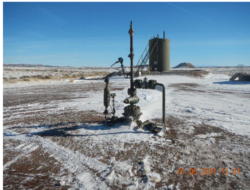
Photo 2. No bradenhead access apparent.
