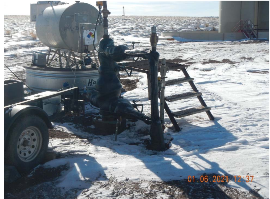
Photo 2. No bradenhead access apparent.
