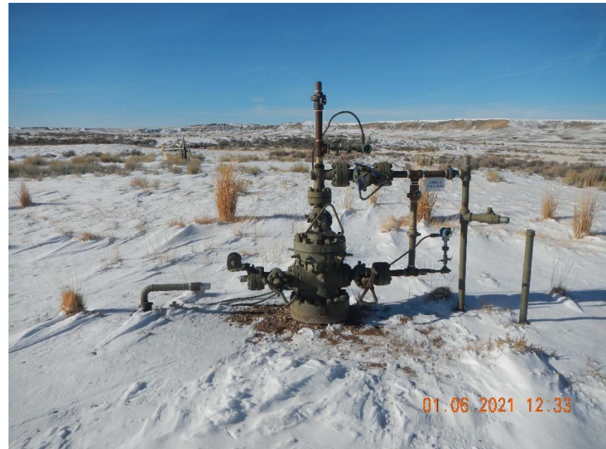
Photo 2. No bradenhead access apparent.
